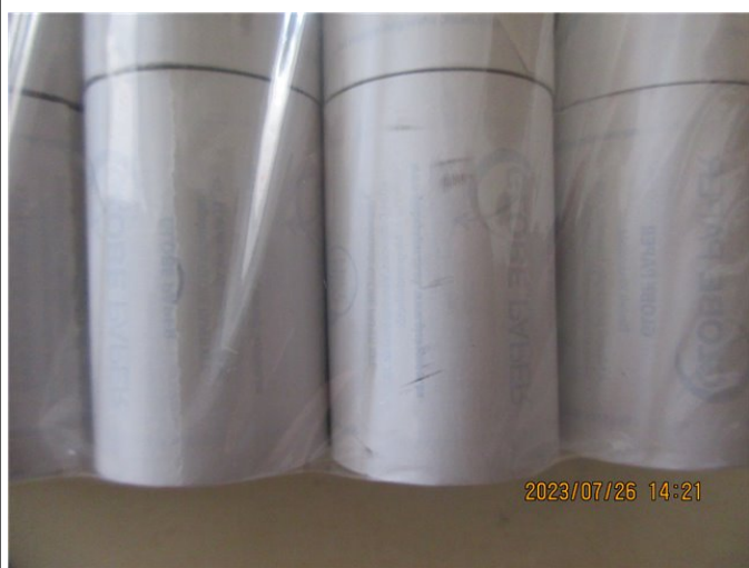
5 - Remark 2. For 48GSM products, There was a slight ink stain on the surface of the product. The factory said the product was so thin that a slight rub would leave ink marks.
