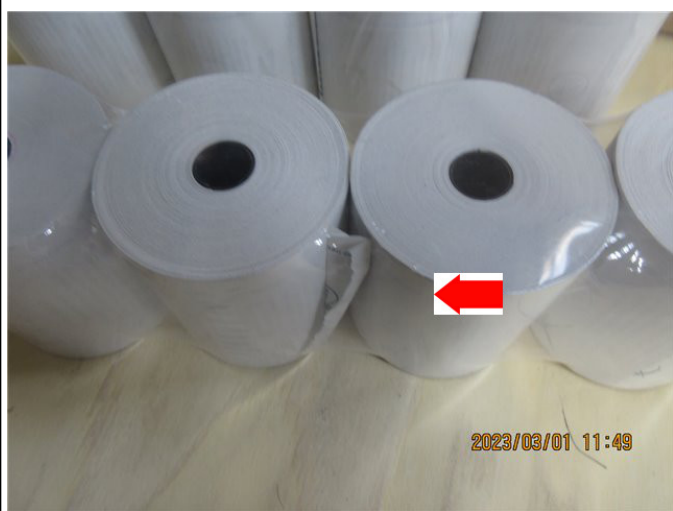
13 - Remark 3, For items 80mmx70mm (55GSM), 80mmx60mm (55GSM) and 80mmx70mm (48GSM). The end of the product was slightly warped.
